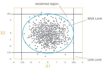
Depending on how the detection threshold is defined, various operations may need to be performed on the trace data. These may be simple, like limit checking or computation of summary statistics. More complex operations like
