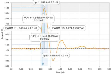
Example waveform, 1kV HBM through short
